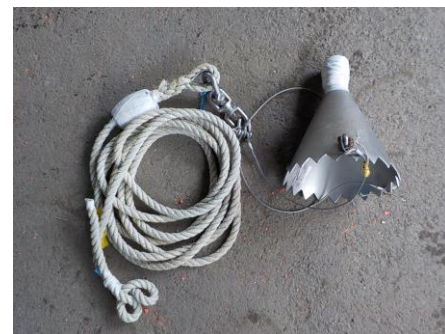
Figure 3. Kumada Dredge sampler
