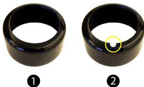
2. Place the sponge wafer in the bottom of the calibration cup and saturate the sponge wafer with approximately 10 mL clean water.
