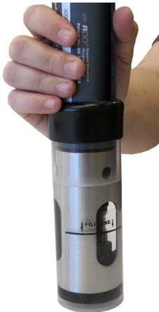
4. Completely submerge the RDO Sensor into the solution.
