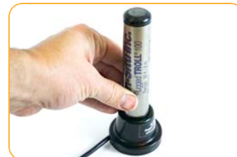
Insert Rugged TROLL in docking station
