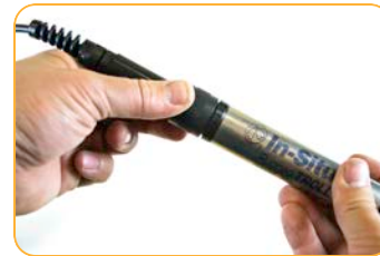
Attach cable to Rugged TROLL.
