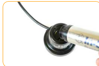
Line up instrument tab with docking station slot.
