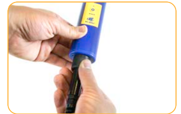
Connect cable to Wireless Rugged TROLL Com.
