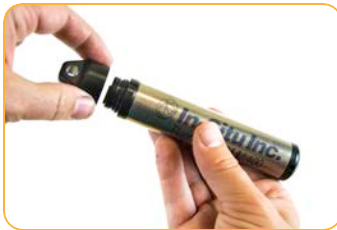
Unscrew cap from instrument.
