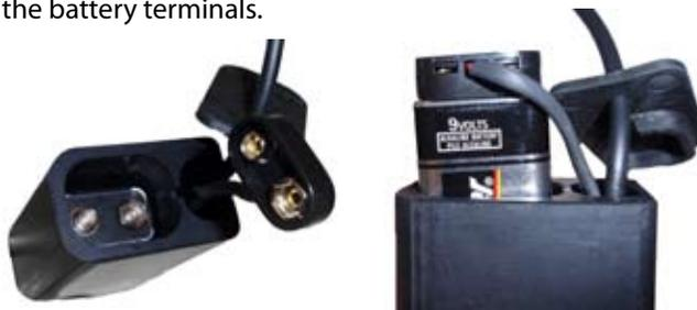
3. Push the battery into the compartment.
